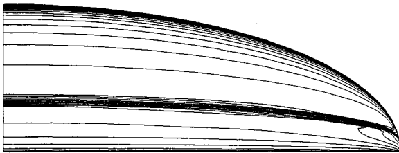
Fig. 6 Surface pressure contours for X_i = 1.0 wing at M_\infty = 0.85 and \alpha = 0 deg (LANS3D).
